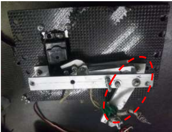
How Servo Horn looks when the parachute door is closed
