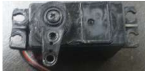
Servo motor for opening the parachute door was retrieved after the crash
