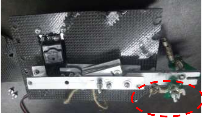
How Servo Horn looks when the parachute door is open
